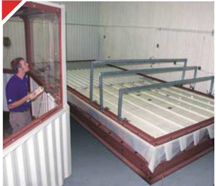
McElroy Metal also has a rigorous testing program to ensure our systems perform as designed in real-life applications. For example, our in-house ASTM E1592 Test Chamber is a valuable asset that enables our engineers to test the wind uplift capabilities of our many systems.
