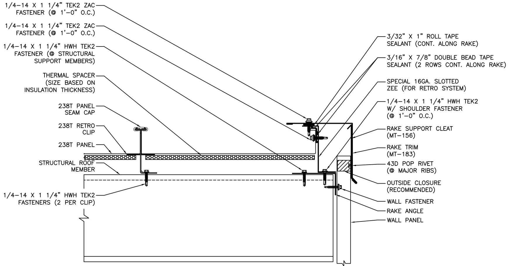
INSULATION REMOVED FOR CLARITY OF DETAIL
