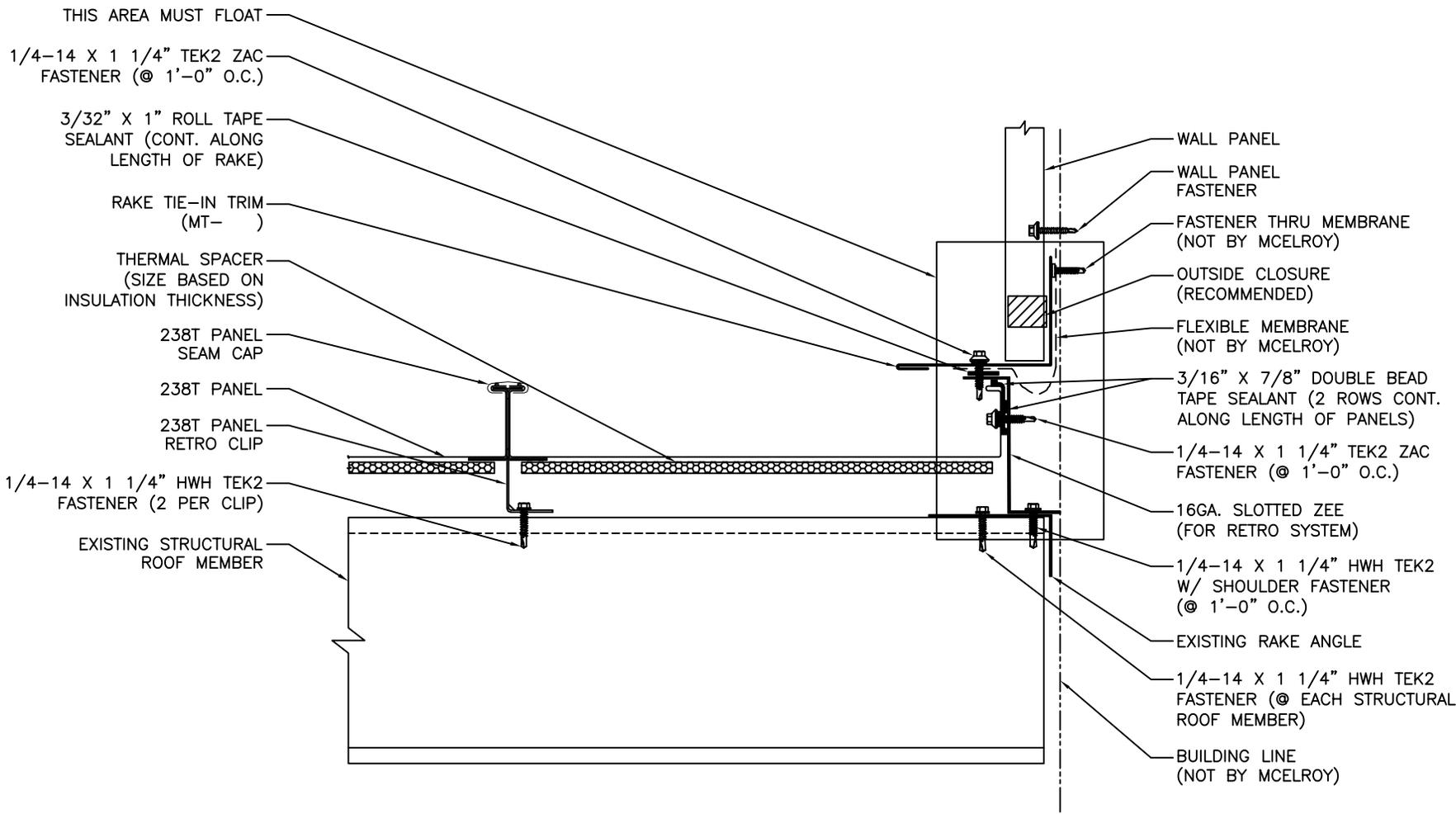
INSULATION REMOVED FOR CLARITY OF DETAIL
