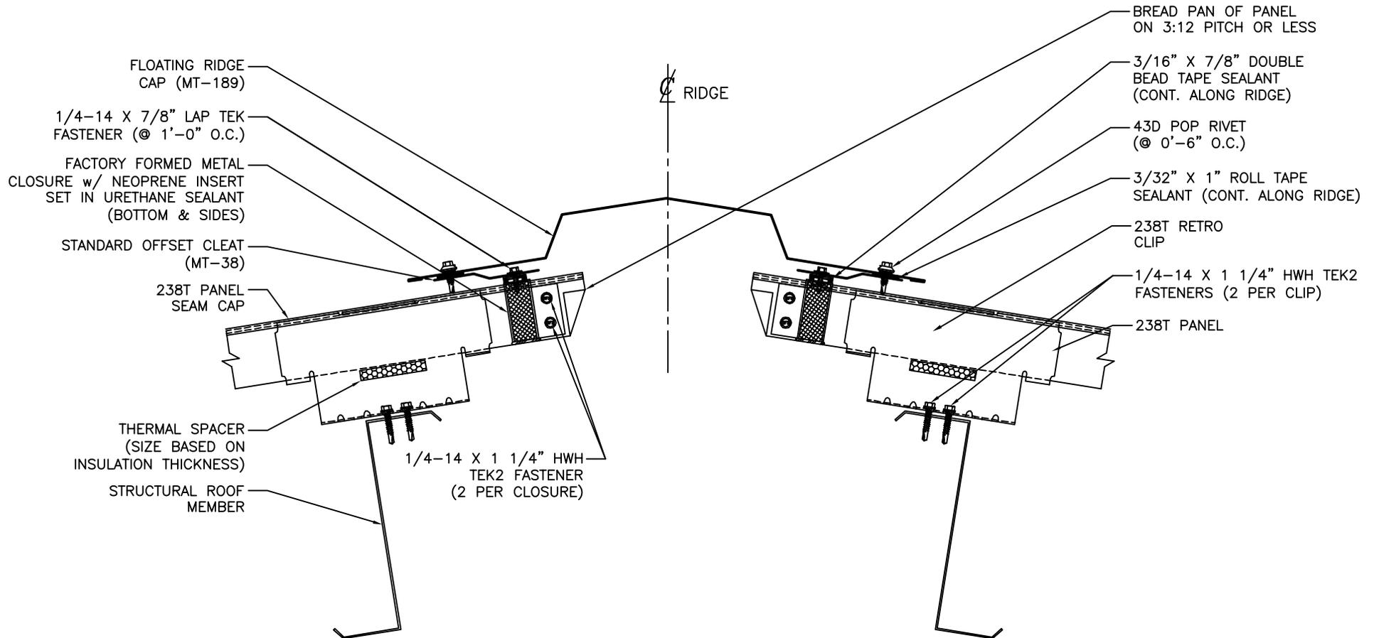
INSULATION REMOVED FOR CLARITY OF DETAIL
