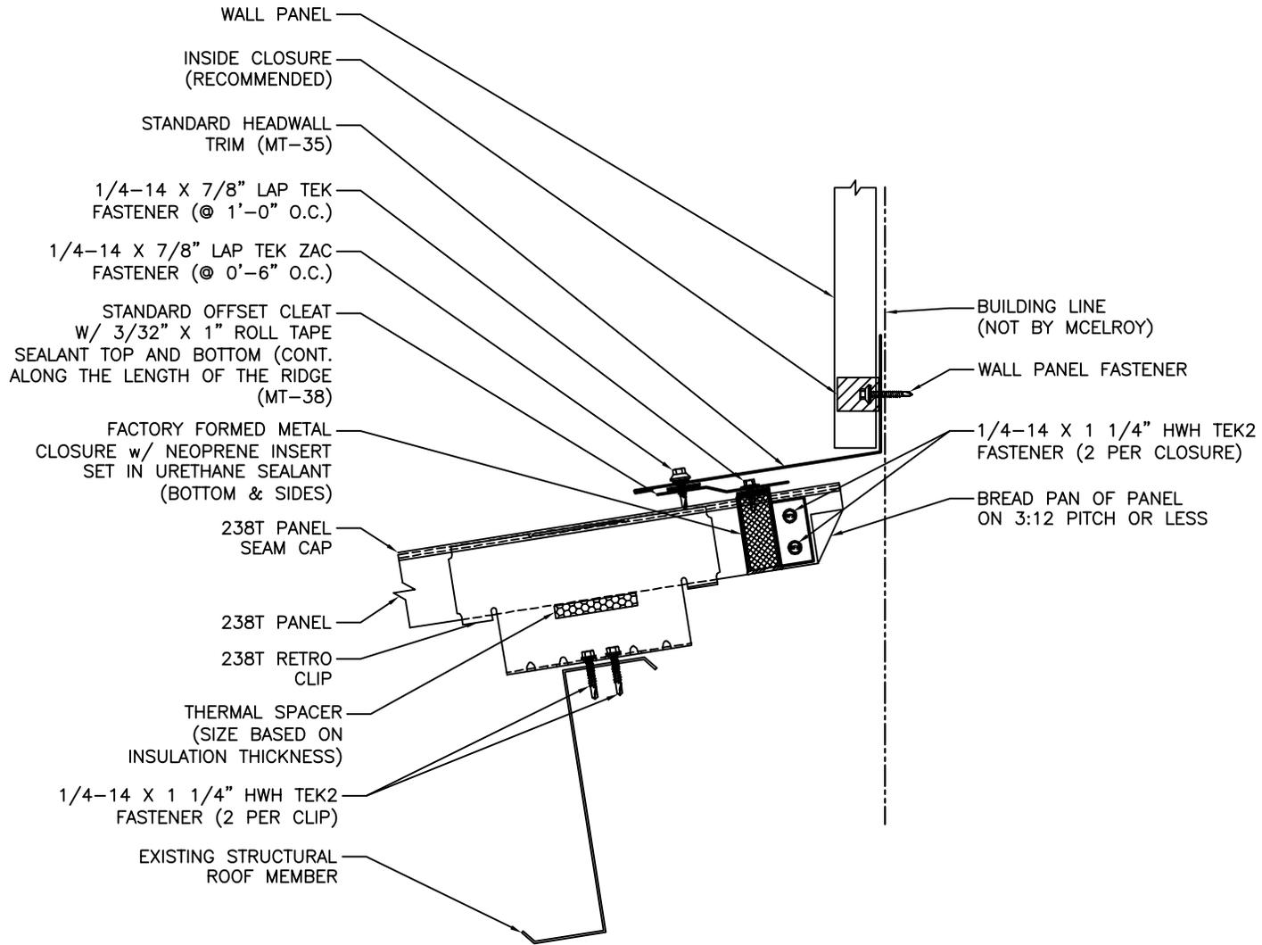
INSULATION REMOVED FOR CLARITY OF DETAIL
