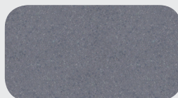
WEATHERED GALVALUME SR:0.30 E:0.79 SRI:27
