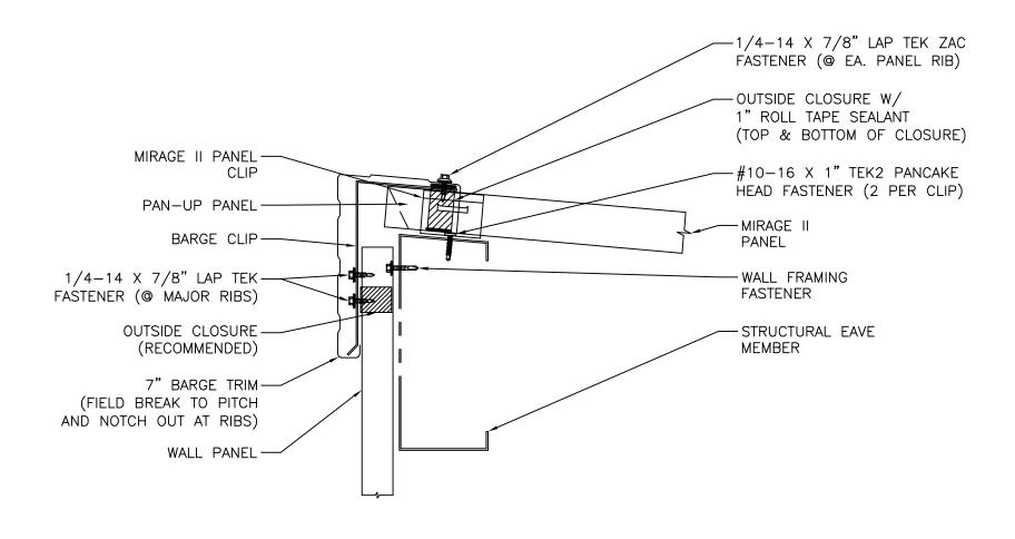
NOTE: WHEN USING 7" BARGE TRIM, INSTALLER MAY USE EITHER BARGE CLEAT OR BARGE CLIP.
