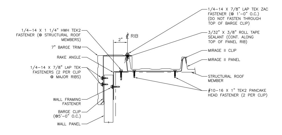
NOTE: WHEN USING 7" BARGE TRIM, INSTALLER MAY USE EITHER BARGE CLEAT OR BARGE CLIP.
