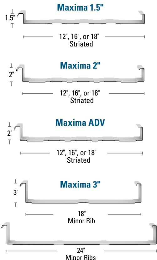
**Note:** Maxima ADV also available without shoulders. Maxima 2" and 3" panels feature a return leg on both the male and female seams. These return legs help create greater strength and uplift capabilities. Maxima 1.5 and ADV do not feature the return legs, which enables the panels to be curved as well as seamed to 180 degrees.
