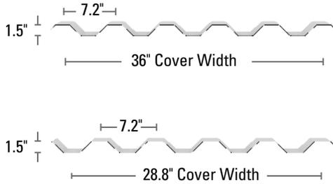
**Note:** Mega-Rib is also available with a 28.8" coverage, which is standard for 26 gauge panels. Please specify if 36" coverage is required.
