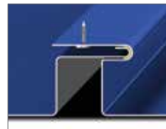
Typical 1 Reveal For 12" Panels
