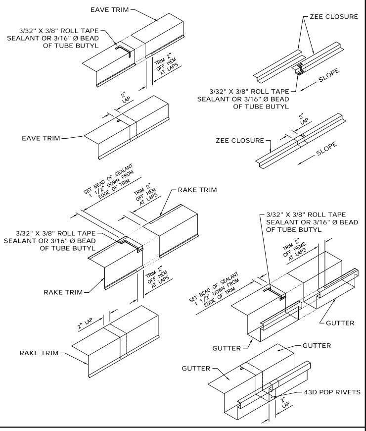
NOTE: 1. Apply specified Roll Tape Sealant or a 3/16" Ø bead of Tube Butyl 1 1/2" back from the edge of the trim. Also, apply a piece of tape sealant or bead of Tube Butyl as a Pigtail to completely seal joint.
