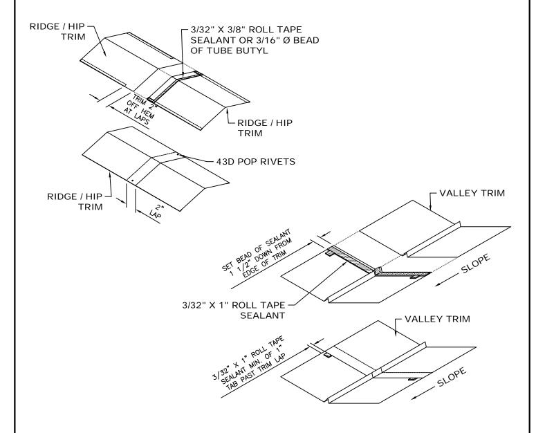
NOTE: 1. Apply specified Roll Tape Sealant or a 3/16" Ø bead of Tube Butyl 1 1/2" back from the edge of the trim. Also, apply a piece of tape sealant or bead of Tube Butyl as a Pigtail to completely seal joint.
