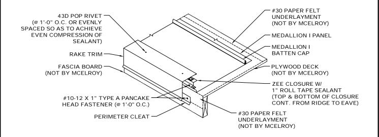
\*NOTE: SOME TRIM ITEMS AND FASTENERS HAVE BEEN REMOVED FOR CLARITY OF ISOMETRIC DETAIL.
