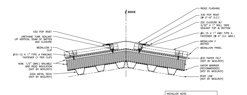
TEMPORARY FASTENER MAY BE REQUIRED TO KEEP PANELS FROM SLIDING DOWNHILL DURING INSTALLATION.
