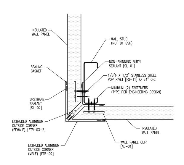
NOTE: FIELD CUT STARTING PANEL AND ENDING PANEL AS REQUIRED AT CORNER TRANSITION.
