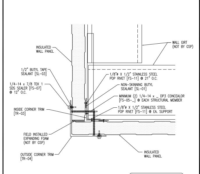
NOTE: FIELD CUT STARTING PANEL AND ENDING PANEL AS REQUIRED AT CORNER TRANSITION.
