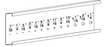
VERTICAL (PERPENDICULAR) SLOTTING ANYWHERE IN WEB OR FLANGE
