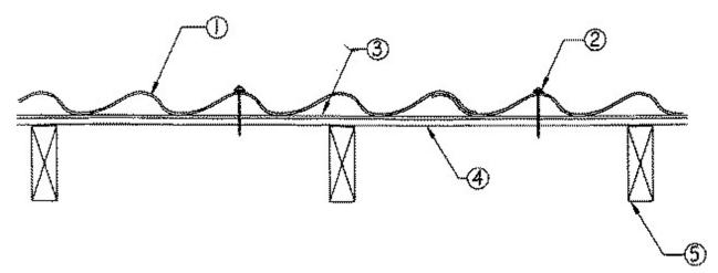
1. Metal Roof Deck Panels\* - Minimum 0.0172 in. thick or 26 MSG coated steel. Max panel width 36 in. **BORGA STEEL INC** (View Classification) — "Classic"
